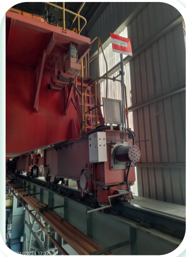
Figure 1: Installation of an automatic retractable rail calliper on the crane
